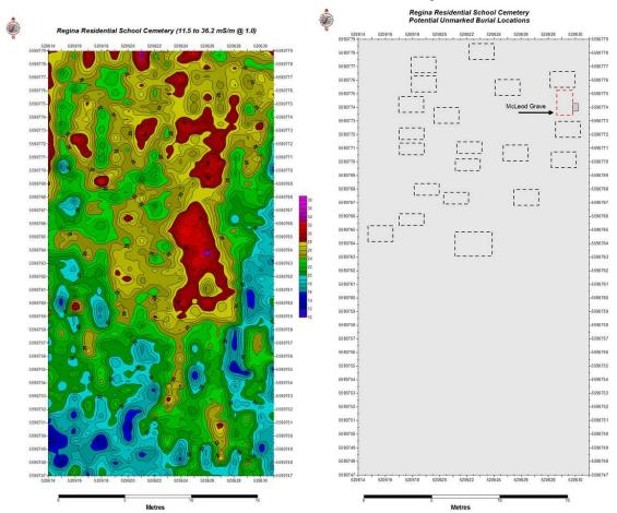
A large amount of blow dirt covers the southern portion of the cemetery. The blow dirt hampers the effectiveness of the EM38 instrument. Further physical work is required to examine that part of the site. The area immediately outside the boundary of the existing fence should also be surveyed since it is possible that the fence may not accurately define the original boundaries of the cemetery.
