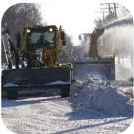
Safety and travel efficiency are provided through the plowing and removal of windrows from in front of **GUARD RAILS** & off of **BRIDGE DECKS**
