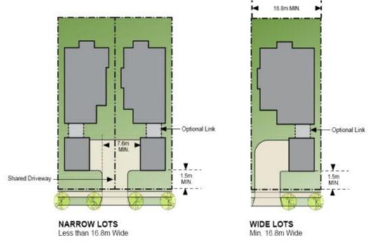
Figure 6C.F8: Garage and Driveway Configuration in the Low-Density Residential Policy Area
