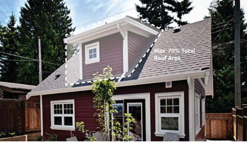
Dormers should be massed to maintain appropriate building and roof proportions, and should occupy no more than 70% of the total roof area (Smallworks Studio).
